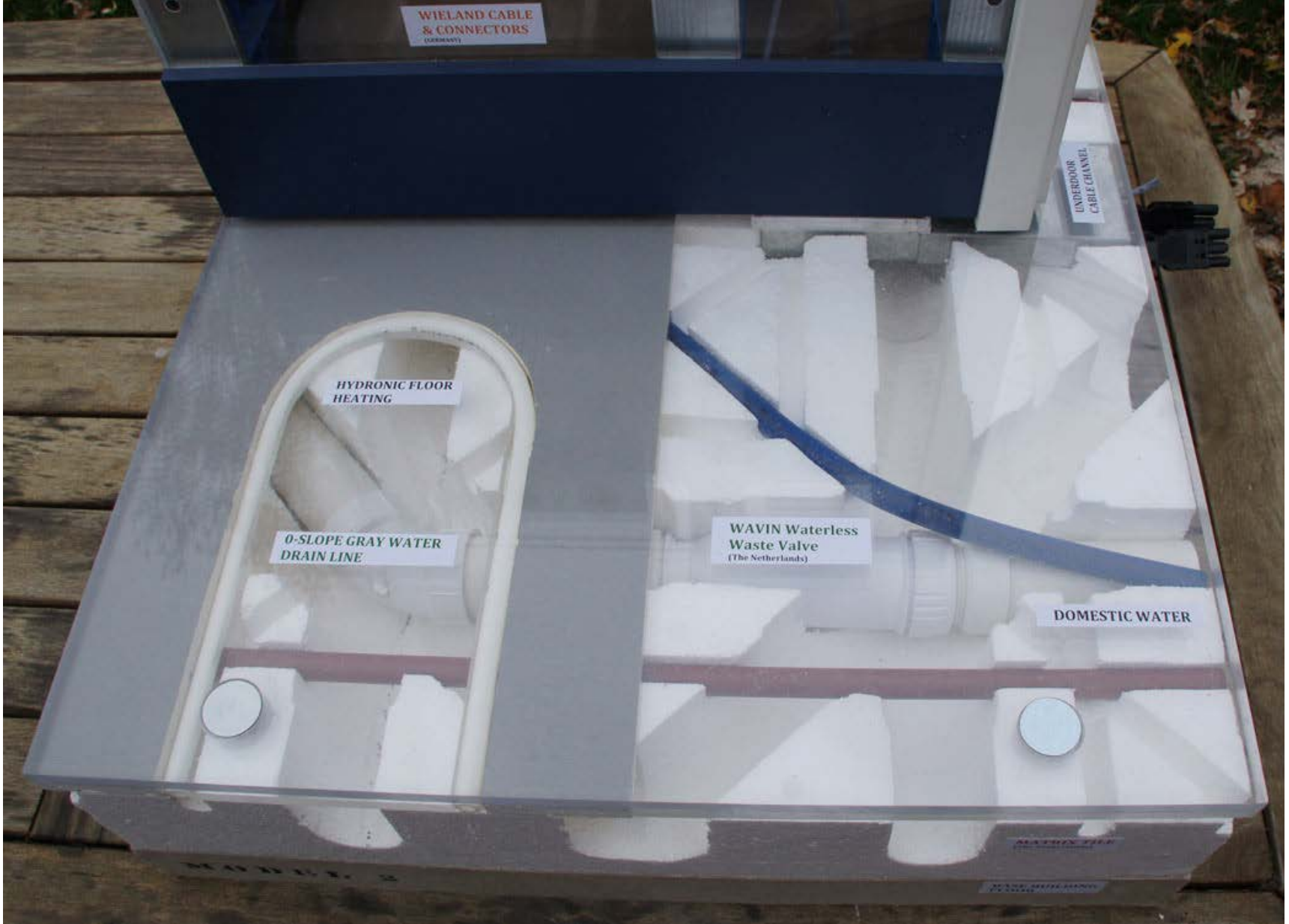
Matrix Tile System, showing 0-slope drain, a waterless waste valve (manufactured by Wavin), domestic water lines, and hot-water floor heating in the bottom-layer of the 2-layer fireproof Matrix-Tile covering.
