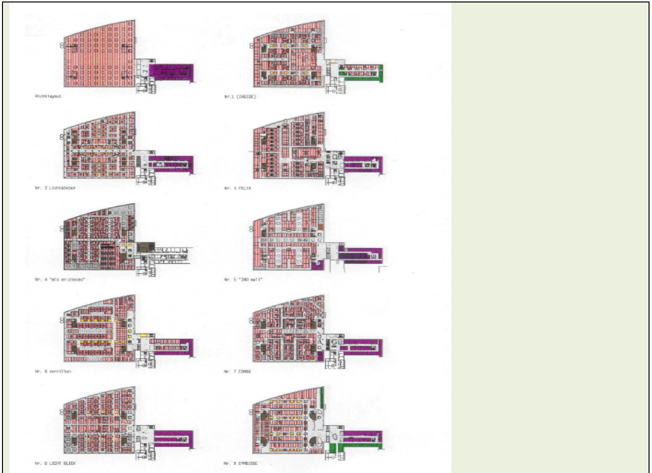
A given floor of the Primary System has the capacity for many secondary system layouts
