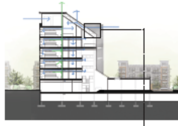
Section showing HVAC
