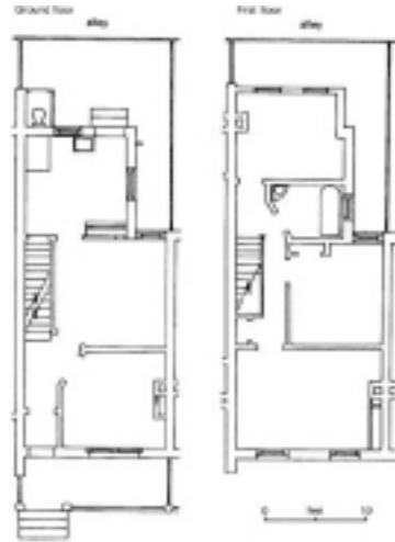
Fig.4 A plan of a Philadelphia mechanic’s house in the early twentieth century, showing a kitchen in the rearmost space, a toilet attached to the back of the house, and a bathroom without toilet on the second floor. (Parish, H.L., One Million People in Small Houses , Philadelphia, 1911.)
