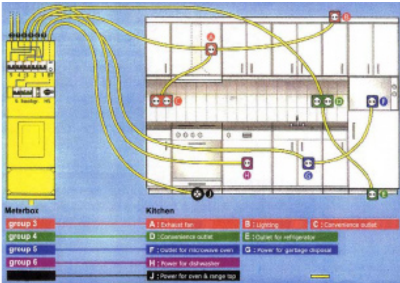
Figure 31: Traditional cabling to the kitchen
